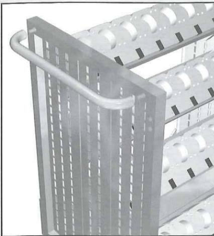
The first step is to attach the handle onto the same side of the transporter where the two swivel casters are located. Use the two supplied M6 bolts, and a 10mm socket wrench. The bolts insert through the holes at the top of the transporter and screw into the thread holes of the handle.
